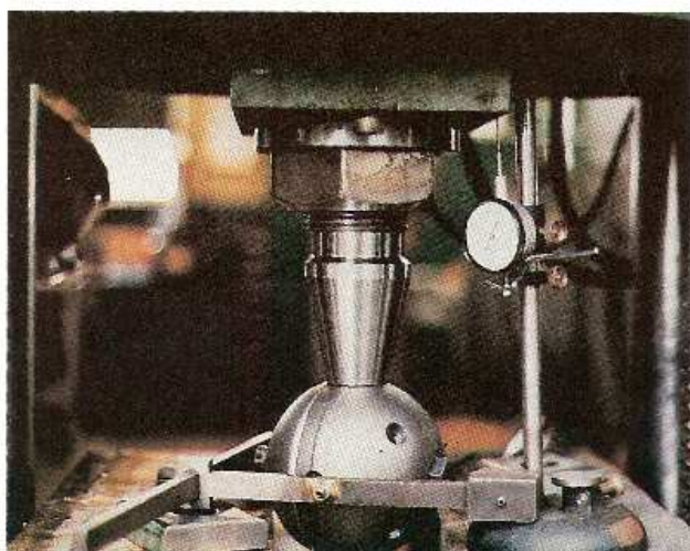
The photo at the left shows actual laboratory testing of the completed forged node.
